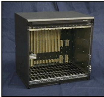
Assembled Backplanes Installed into Enclosures
